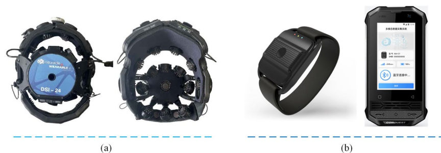
Fig. 2 Photos of devices used for signal data collection. (a) Wireless dry electrode EEG device DSI-24. (b) Intelligent wristband ES1 used for GSR and PPG data acquisition.
